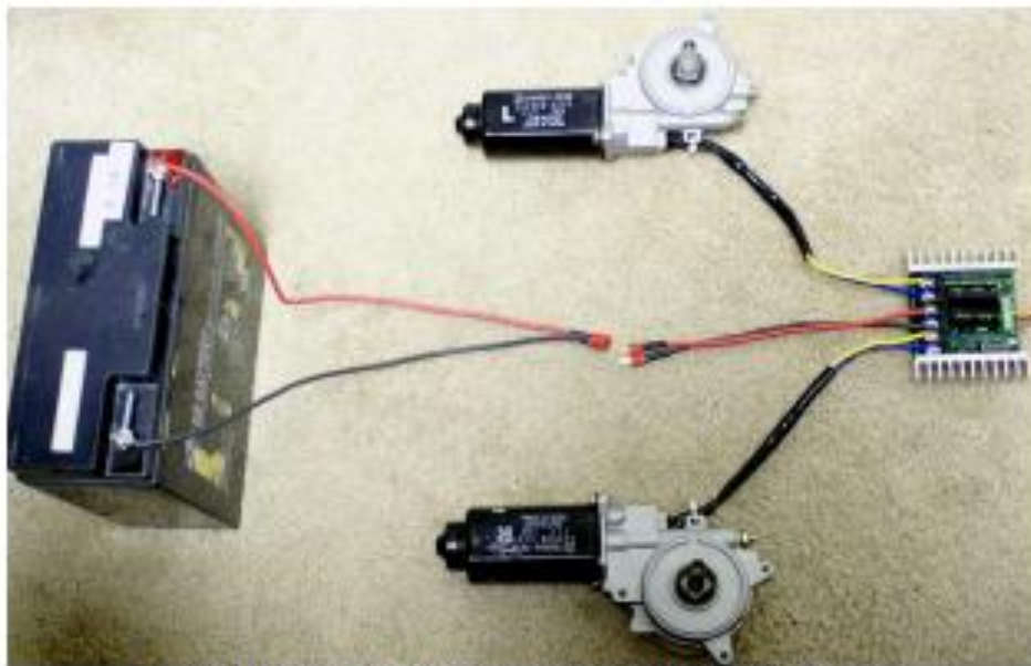
Using a battery connector to connect/disconnect power to Sabertooth
