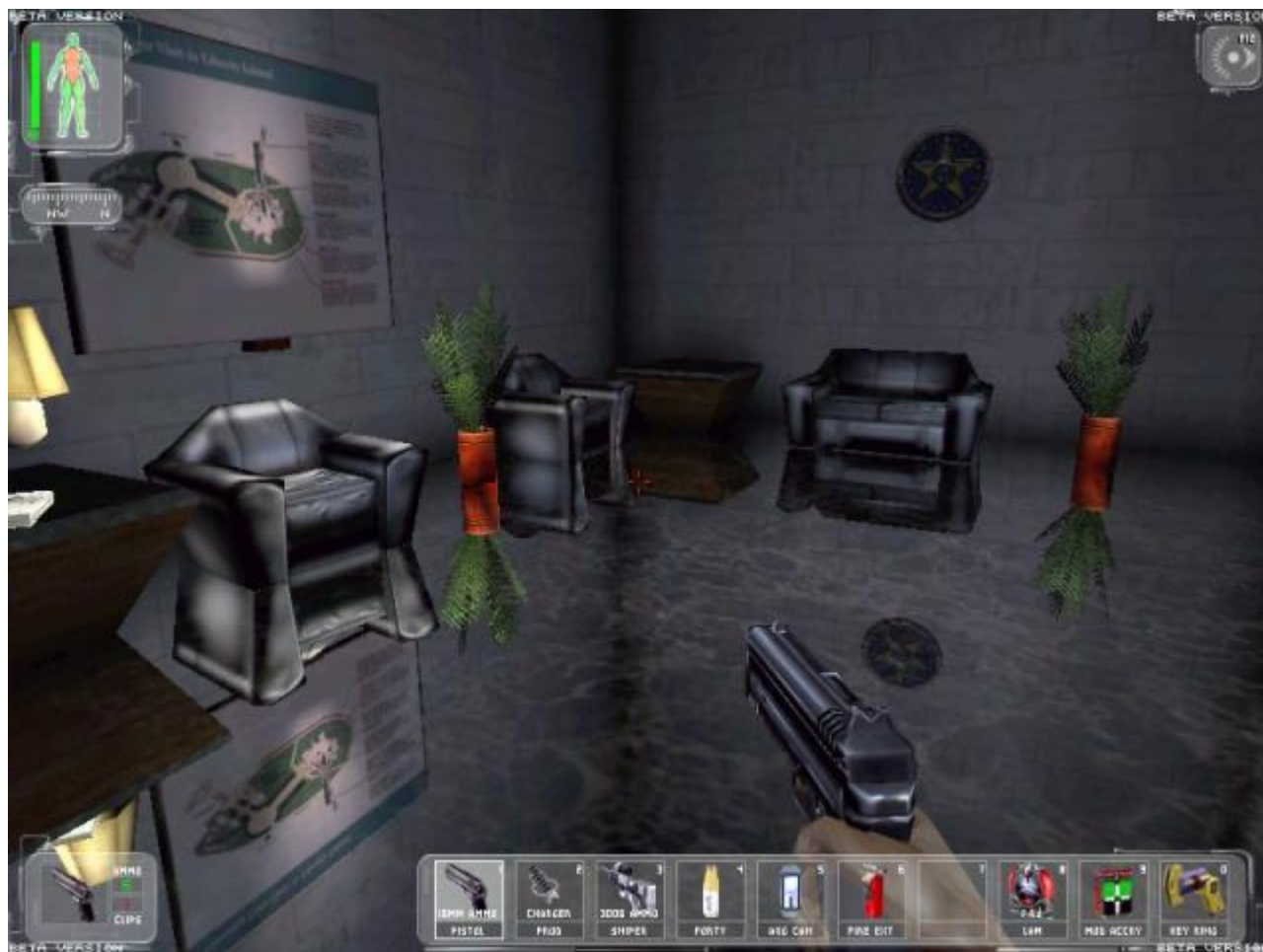
Figure 6-31. Reflections in Deus Ex (Ion Storm Austin / Eidos Interactive, 1999). The polished stone floor appears reflective, but it’s actually semitransparent, and there’s another, duplicated, upside-down version of the same room underneath.
