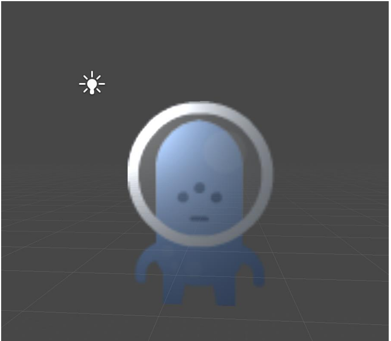
Figure 5-12. A sprite using the Diffuse shader; it's now shaded and responds to light.
