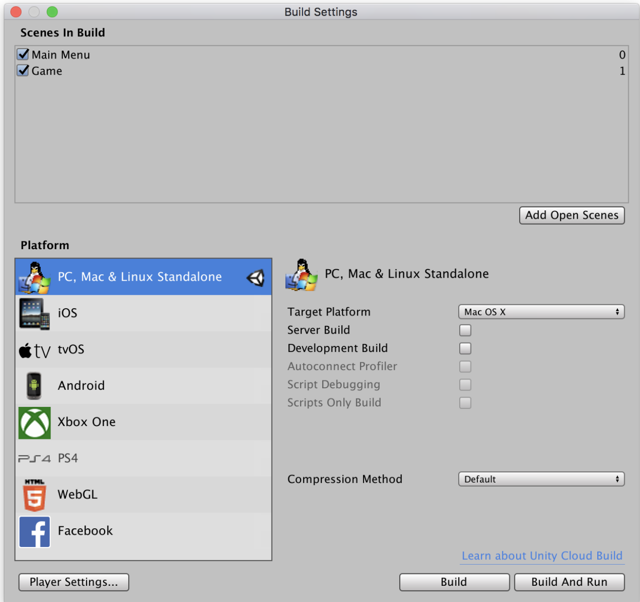
Figure 2-4. The scene list in the Build Settings screen, with two scenes added. A scene must be in this list in order to be loaded.
