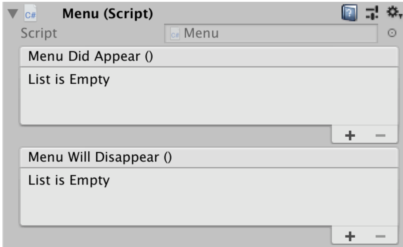
Figure 9-8. The Menu Did Appear and Menu Will Disappear events, to which you can add function calls.
