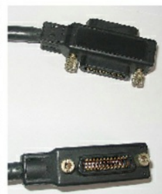
Figura 1.2 Interfaz GPIB. National Instruments de México®
