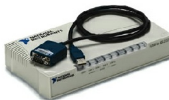
Figura 1.1 Interfaz RS232. National Instruments de México®
