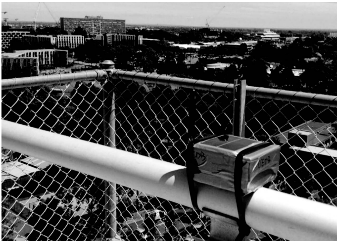
Figure 7.11 One sensor node with solar energy harvesting deployed at Monash University Clayton campus.
